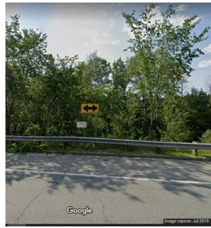
NHDOT removed the streetlight and downgraded the warning sign sometime between 2008 and 2019. Replacement of these safety devices, moving the guardrail back to improve the sight distance from NH 117, and signage for drivers approaching the end of NH 117 may all help improve safety in this location.
